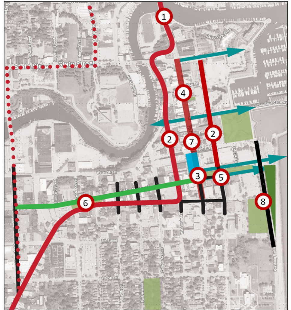
Figure 1: Overall design concept for downtown Racine, WI. 1) Connecting State Trunk Highway re-designation to Wisconsin Avenue at 2nd Street; 2) Two-way Wisconsin and Lake Avenues; 3) Begin Monument Square studies and detail design; 4) Main Street road diet; 5) Bicycle lanes on 6th Street, east of Main Street; 7) Monument Square reconstructed as a plaza; and 8) Reconstruct Pershing Park Drive concurrent with waterfront development. Note the blue lines with arrows are important views that need protecting. The dotted line represents an alternative re-routing option for the State Trunk Highway.
